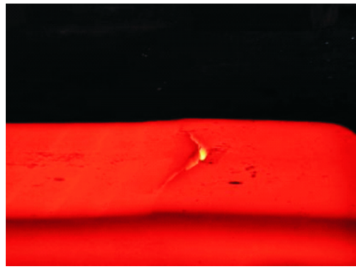
图 1 N08120 钢锭初锻开裂的宏观形貌图 Fig. 1 Macroscopic morphology of crack on N08120 steel ingot after primary forging
